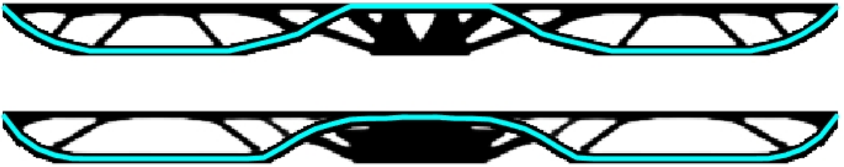
Fig. 15 The effect of self-weight on the optimization of a two-span beam. Top: without self-weight and T_{pre} = 0.8 \times T_{STD} ; Bottom: with dominant self weight and T_{pre} = 50 \times T_{STD} . When self-weight is dominant, material is more concentrated near the central support so that deformation due to self-weight is reduced.
