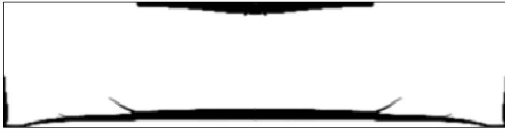
(b) Optimized layout with V = 0.1 and \delta = 0.002 . 300 design iterations with gradual refinement.
