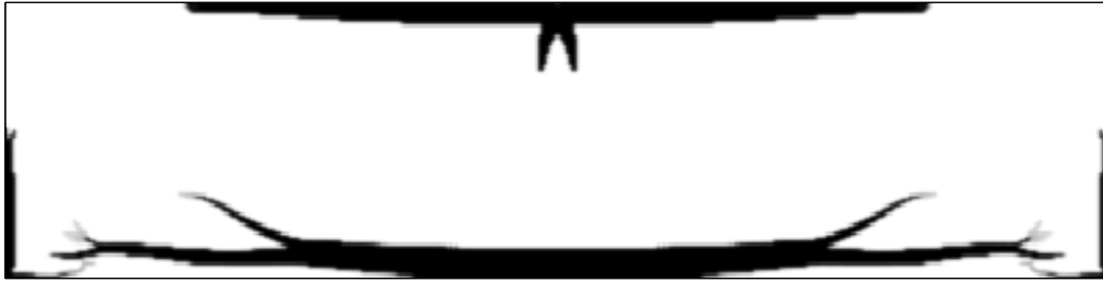
(a) Optimized layout with q = 1 , 200 design iterations with p_E = 3, p_\alpha = 3, p_{\sigma_y} = 3 and filter radius r = 0.015 .
