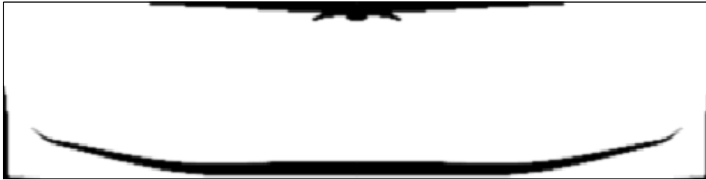
(b) Optimized layout with q = 2 , 200 design iterations with p_E = 3, p_\alpha = 3, p_{\sigma_y} = 3 and filter radius r = 0.015 .
