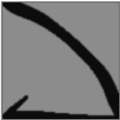
(b) Optimized layout after 500 design iterations, 80% concrete, 20% steel. Black = steel, gray = concrete.
