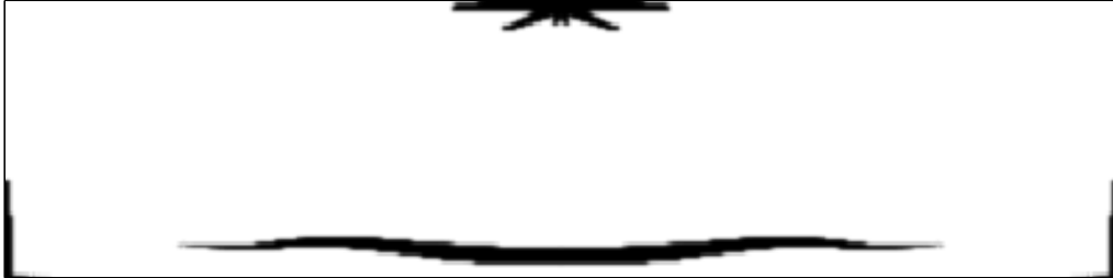
(a) Optimized layout with V = 0.05 and \delta = 0.001 . 200 design iterations with p_E = 3, p_\alpha = 3, p_{\sigma_y} = 3 and filter radius r = 0.015 .
