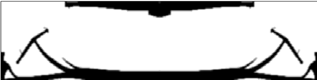
(c) Optimized layout with V = 0.2 and \delta = 0.005 . 150 design iterations with gradual refinement.
