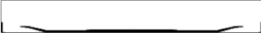
(c) Optimized layout with q = 4 , 150 design iterations with gradual refinement.
